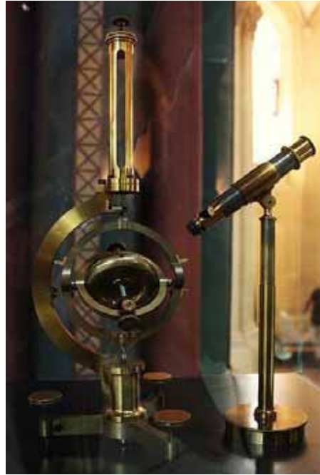
Fig. 3.13: Conventional gyroscope, invented in 19 th century by Leon Foucault [39]
